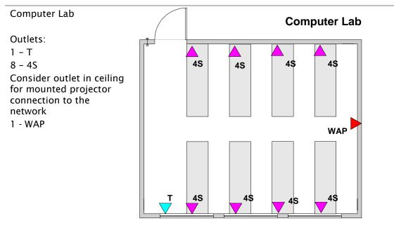
Sample outlet recommendations for rectangular back- to- back stations computer lab configuration:
